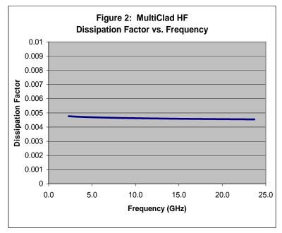
**Figure 2** demonstrates the Stability of Dissipation Factor across Frequency. This characteristic demonstrates the inherent robustness of Arlon Laminates across Frequency, providing a stable platform for high frequency applications where signal integrity is critical to the overall performance of the application.
